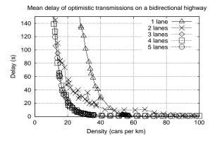
Figure 4: Optimistic delay on bidirectional highways with 1 to 5 lanes in each direction
