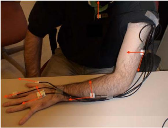
**Figure 1** Sensor setup and orientation of the axes of the accelerometers.
