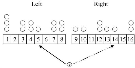
Fig. 1. The 2-left scheme. A newly inserted item, labeled  $z$ , is placed in the less filled of two random buckets, one from the left and one from the right. Ties are broken to the left. A search for  $z$  may require searching both of the buckets in which  $z$  might have been placed.
