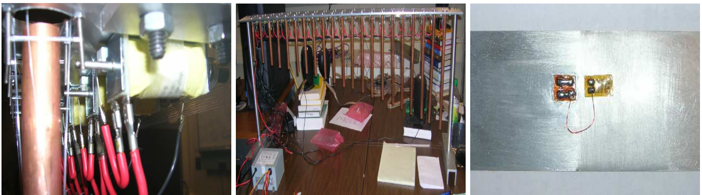
Fig. 6. An array of 24 digital hammers, developed by PhD candidate Georgios N. Lilis, MEng student Sining Qi and undergraduate student Jae-Hoon Lee. Each hammer (left) consists of a piece of metal with a coil wrapped around it. When a current is passed through the coil, a magnetic field is created that causes the hammer to displace from its rest position; a simple circuit with a digital interface controls the current flow from an external power source. A simple demo of this tool is a musical instrument: each hammer hits a pipe of different length, thus producing different sounds (middle). Our goal however is to demonstrate another application of the dWFS concept: here, in conjunction with strain sensors (right), we can synthesize small pressure waves inside an object by having the hammers tap on its surface, and then map these waves at other surface points using strain sensors, to create a tomographic picture of the object's interior without destroying it.
