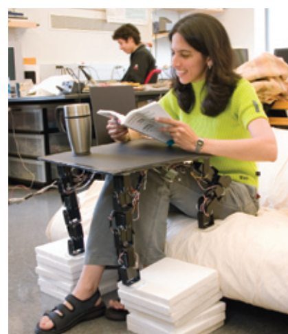
The "balancing table" built in Nagpal's lab, an example of a multi-agent system that converges towards the right answer (or in this case, staying upright). "The table idea is actually just one possible way to think about this concept," explains Nagpal. "Another is a bridge, or a programmable assembly surface on which you could move objects. Just think of a surface made up of several of these 'table-like' panels connected in an array. In that way our original idea for a self-balancing chain has evolved not into just a table, but into a more general 'self-adaptive structures' concept."
