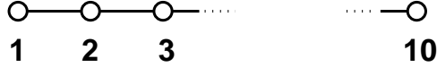
Figure 4: Network topology used in the experiments. An edge between two nodes indicates that they are within radio range. The leftmost node generates the data, and the rightmost node receives it.
