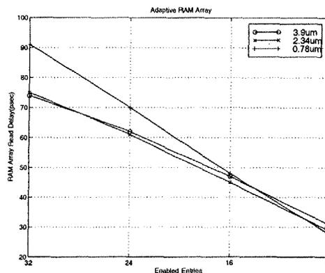
Figure 8: Adaptive RAM array delay values
