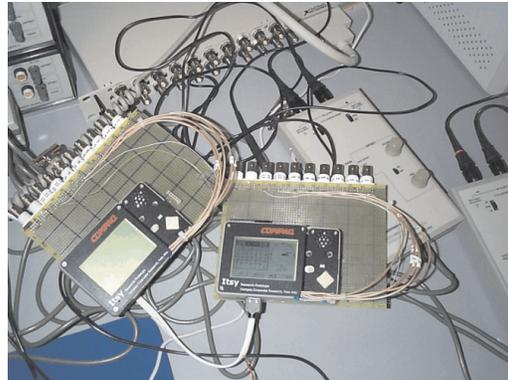
Figure 1: Equipment setups used to measure power.
