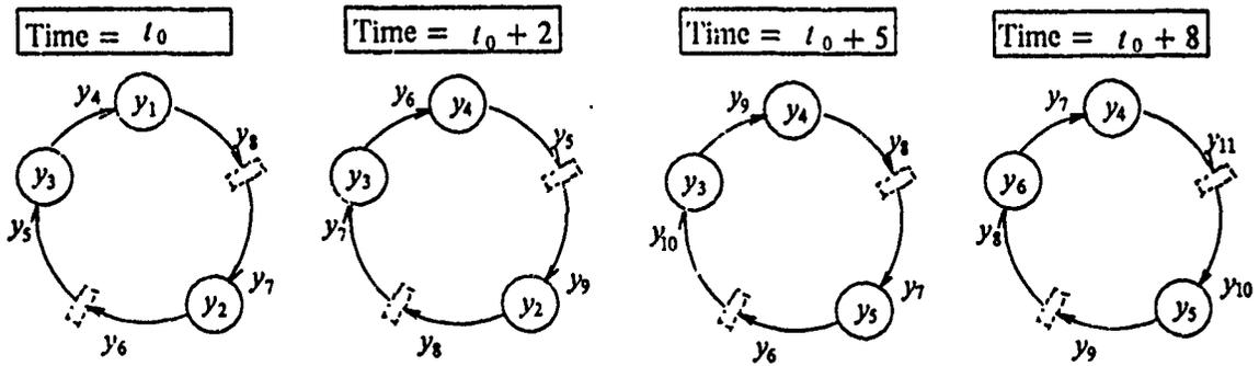
Figure 4-3: Defective systolic ring with 2 faulty cells
