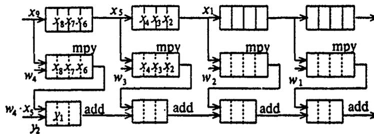
Figure 2-4: Two-level pipelined systolic array for convolution, using pipelined arithmetic units of Figure 1-1 (b)
