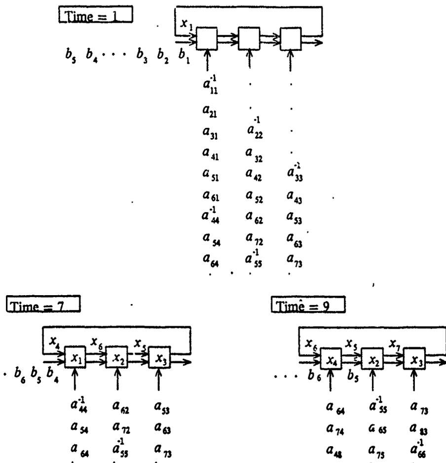
Figure 4-4: Systolic ring for solving triangular linear systems
