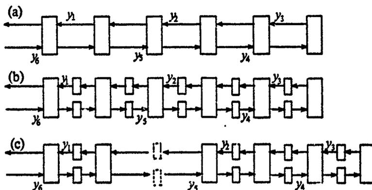
Figure 4-1: Linear array with feedback: (a) original array, (b) reduced throughput and (c) single failure
