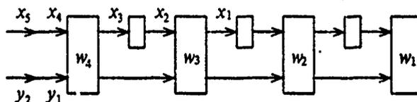
Figure 2-1: Uni-directional linear systolic array for convolution
