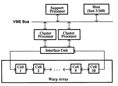
Figure 1: The Warp architecture.
