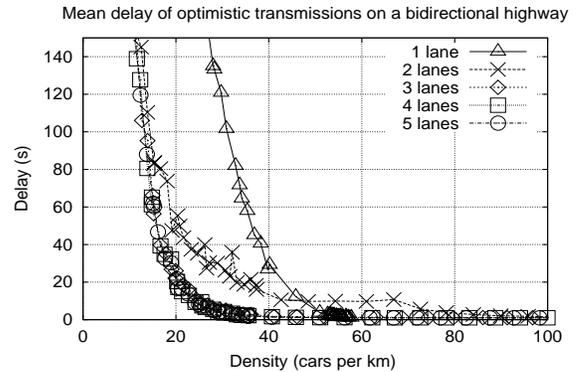
Figure 4: Optimistic delay on bidirectional highways with 1 to 5 lanes in each direction
