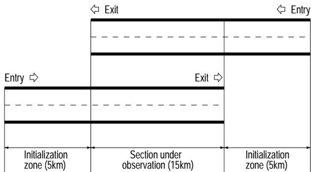
Figure 1: Highway geometry used by the traffic simulator of this paper
