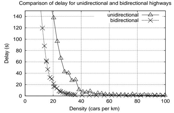
Figure 3: Optimistic delay on unidirectional and bidirectional highways with 5 lanes in each direction
