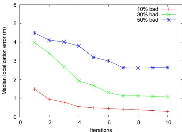
Figure 7: Iterative refinement of localization solutions by gradually decreasing  $\tau$  gives improved accuracy. Each curve is a separate experimental condition, differing in the percentage of nodes in the population with ranging errors of 50% (10%, 30%, 50% bad nodes).
