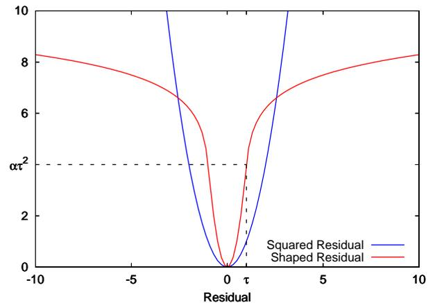
Figure 2: A comparison between the standard squared residual used in conventional least squares and our shaped residual, as in Eq (3) with  $\alpha = 4$ ,  $\tau = 1$  and with  $u$  and  $v$  as defined in (4) and (5). Note that the shaped residual function is shaped like a "U" near 0 and like "wings" for values larger than  $\tau$ .
