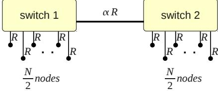
Figure 3: A two-rack network topology from Scenario 2. Two groups of  $N/2$  nodes each connect to a non-blocking switch via rate  $R$  links. The inter-switch link runs at a different rate,  $\alpha R$ , where  $\alpha$  is a constant typically greater than 1.
