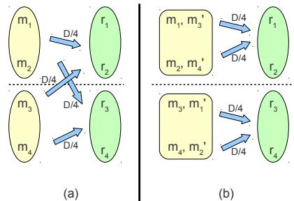
Figure 8: Map task assignment with (a) no redundant mappers, and (b) redundant mappers. Redundant mapper of primary mapper  $m_i$  is indicated as  $m'_i$ . The dotted line represents the rack boundary. In both cases the same total amount of data,  $D$ , is moved to reducers. Note that in (b), no flows cross the rack boundary.
