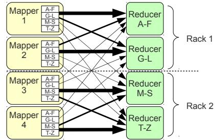
Figure 7: Data-flow diagram for a MapReduce sort run. Thickest arrows represent the fastest, node-local flows where no network is used. Medium-thick arrows represent fast, rack-local flows. Thin arrows represent slowest, cross-rack flows.
