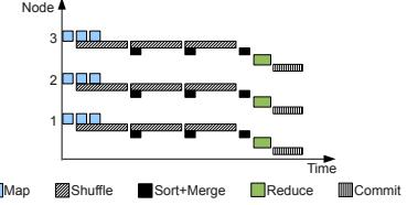
Figure 1: Hadoop job progress occurs over multiple nodes in sequential phases: map, shuffle, sort+merge, reduce, and commit.
