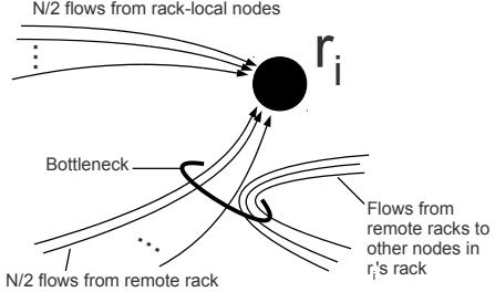
Figure 4: Diagram accompanying the analysis for Scenario 2. The flows shown correspond to the baseline case without speculative redundant computation.
