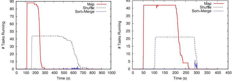
Figure 9: Progress of sort jobs on Configuration A (left) and Configuration B (right). The vertical axis shows the number of running tasks belonging to one of the MapReduce phases.
