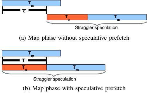
Figure 2: A comparison of a map phase without (a) and with (b) speculative prefetch.
