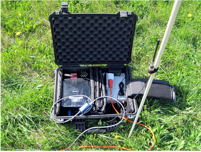
Fig. 9. GNURadio USRP2 sensor deployed in the field, along with the host PC used to record the measurements.
