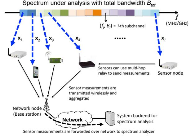
Fig. 1. A wideband spectrum (*e.g.*,  $B_{tot} \approx$  a few GHz) under analysis is partitioned for collective measurement efforts by multiple sensor nodes. Spectral analysis on the measured data takes place at the potentially distant system backend.
