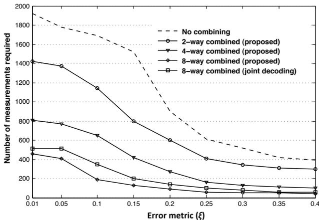
Fig. 8. Total number of measurements used in spectrum analysis vs. accuracy of decoding measured by error metric  $\xi$ . The proposed methods run 2 refinement stages. Joint decoding for 8-way combined uses a comparable number of measurements to the proposed 8-way combined for similar error performance, but joint decoding is much harder computationally and takes significantly longer decoding time (see Section V.A).
