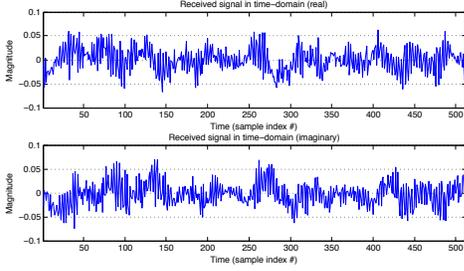
Fig. 3. Time-domain representation of a real wireless spectrum (source: 512 samples from 6-MHz bandwidth UHF Ch. 21 at  $f_c = 515$  MHz measured in Cambridge, MA on Saturday May 21, 2011 11:03pm EST, using USRP2)
