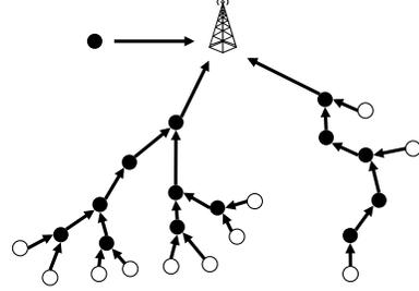
(b) Network nodes (in black) relay measurements of other network or sensor nodes
