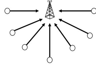
(a) Sensor nodes (in white) transmit measurements directly to base station
