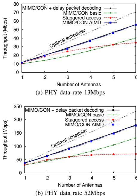
Fig. 4: MIMO/CON throughput with 20 users in simulations.
