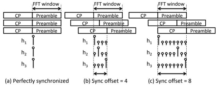
Fig. 2: Use of cyclic prefix (CP) to tolerate synchronization offsets among senders. Synchronization offsets cause an increase in the number of unknowns in CSI.
