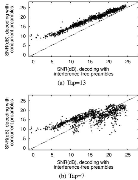
Fig. 3: MIMO decoding performance in  $4 \times 4$  MIMO. Each dot represents a MIMO packet decoded by two different CSI estimated from concurrent preambles and sequential preambles. Dots above the 45-degree line mean that using CSI from concurrent preambles yields higher decoded packet SNR.
