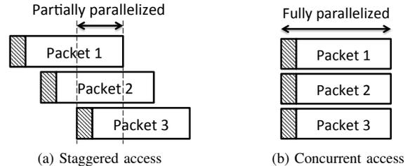
Fig. 1: Two access strategies for multiuser MIMO networks. Shaded areas denote packet preambles: (a) conventional staggered approach and (b) concurrent approach of this paper.
