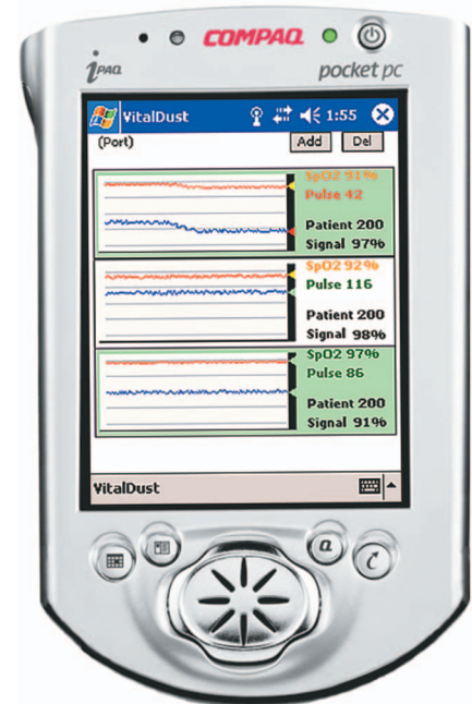
Figure 3. PDA-based multiple-patient triage application. The screen shows real-time vital sign (heart rate and blood oxygen saturation) data from three patients.
