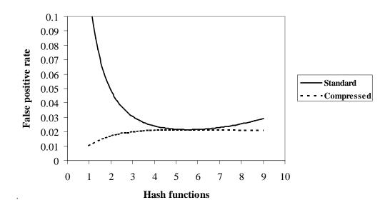
Figure 1: The false positive rate as a function of the number of hash functions for compressed and standard Bloom filters using 8 bits per element.
