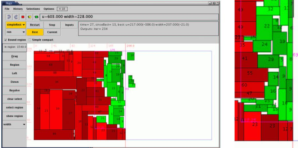
Figure 1: Interactive system: The image on the left is a screen shot of our system in use. The user has selected a region to apply BLD\* to and has frozen most of the rectangles (frozen rectangles shown in red/dark gray, unfrozen in green/light gray). The image on the right shows a blowup of the selected portion of the packing, after BLD\* has run for a few seconds and the user has pressed the Best button to see the best solution found.
