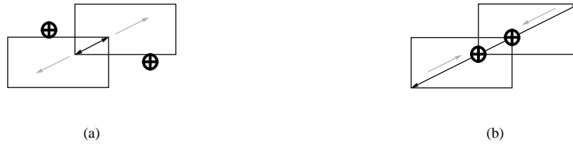
Figure 7: Computation of overlap vectors in Hirsch's algorithm. The configurations in (a) and (b) have identical overlap regions, but the overlap vectors must be calculated to cause movement in different directions due to the relative placement of the overlap and the points.
