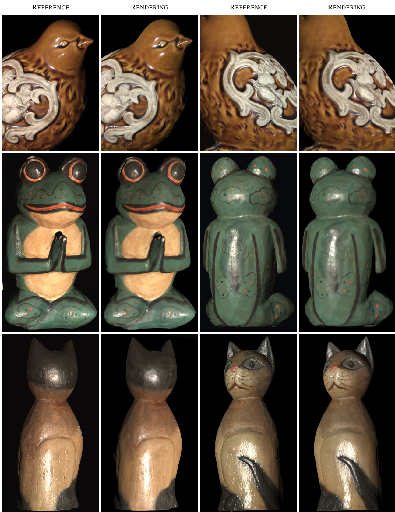
Figure 12: Rendered images computed using models captured by our scanner compared to reference images. The chosen light and view positions are approximately 20 degrees away from the closest measurement location. Note that we do not attempt to render shadows.
