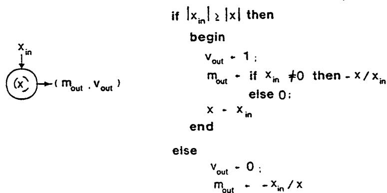
Figure 3. Cell definitions for a triangular systolic array for performing triangularization with neighbor pivoting.
