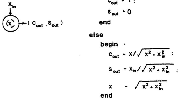
Figure 4. Cell definitions for a triangular systolic array for performing orthogonal triangularization with Givens rotations.
