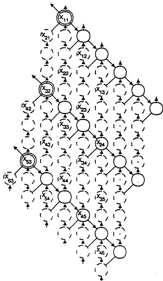
Figure 6. Systolic array for triangularizing a band matrix.
