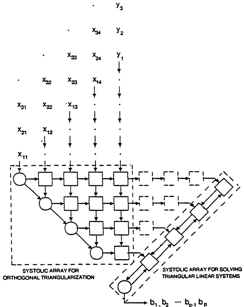
Figure 5. On-the-fly least squares solutions using systolic arrays.
