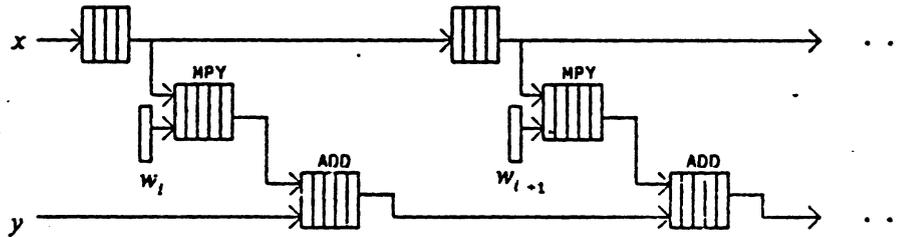
Figure 5. Two-level pipelined systolic array for 1-D convolution
