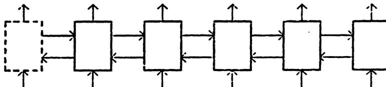
Figure 16. Bi-directional systolic array with a boundary processor
