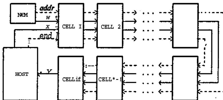
Figure 15. I/O interface of the Warp processor when performing FFT
