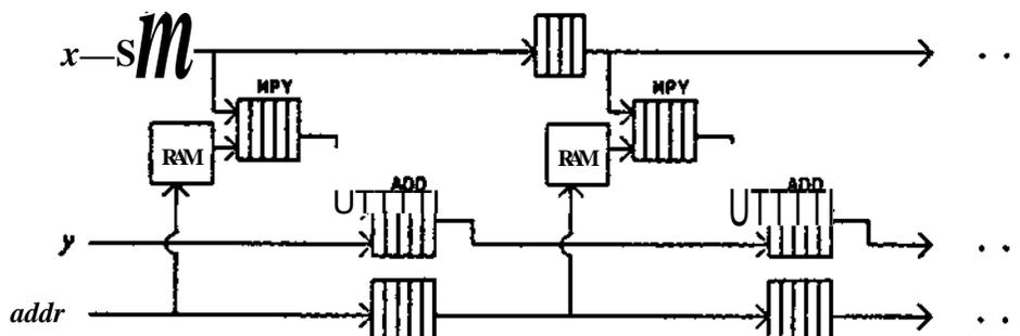
Figure 6. Systolic array using adaptive weights for interpolation and resampling
