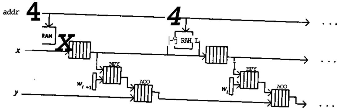
*Figure 8. Another two-level pipelined systolic array for two or higher dimensional convolutions*
