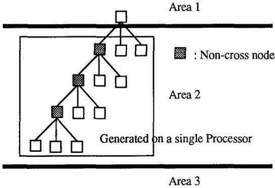
Figure 8: In stage 1, any non-cross node's ancestors in area 2 must have been generated on the same processor.
