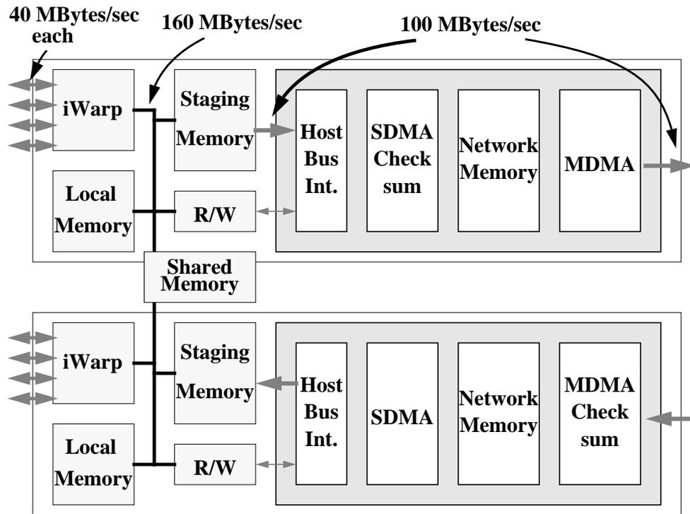
Figure 7: Block diagram iWarp network interface
