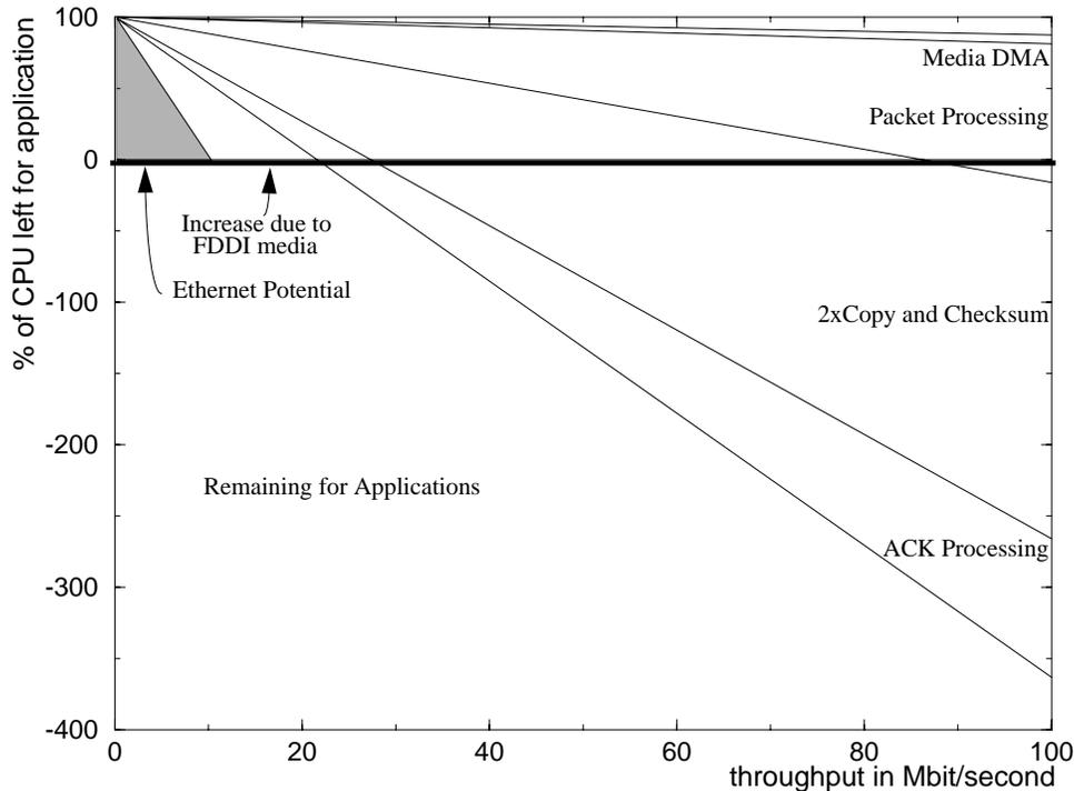
Figure 10: Overhead for Communication over FDDI
