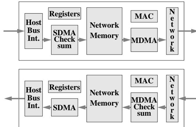
Figure 5: Block diagram generic network interface
