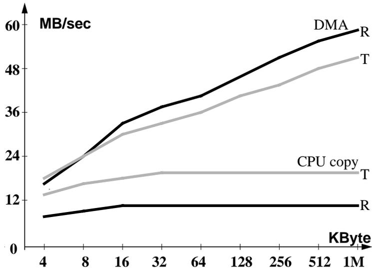
Figure 9: Transmit (T) and receive (R) transfer rates across TURBOchannel
