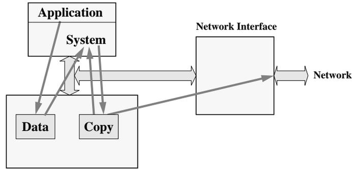
Figure 2: Dataflow in traditional network interface
