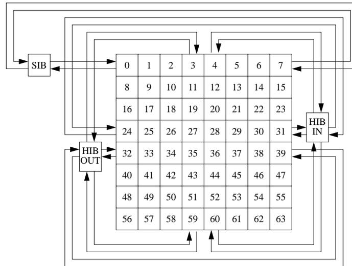
Figure 6: Connecting the network interface to iWarp
