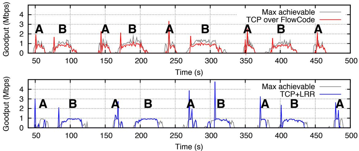
Fig. 6: Measured goodput as compared to the maximum achievable over emulated flights. Each burst of delivery occurs in the correspondingly labeled region of the flight path (see Figure 5). *Top*: TCP over FlowCode, using four Tx’s and four Rx’s. *Bottom*: TCP+LRR, using one Tx and one Rx.
