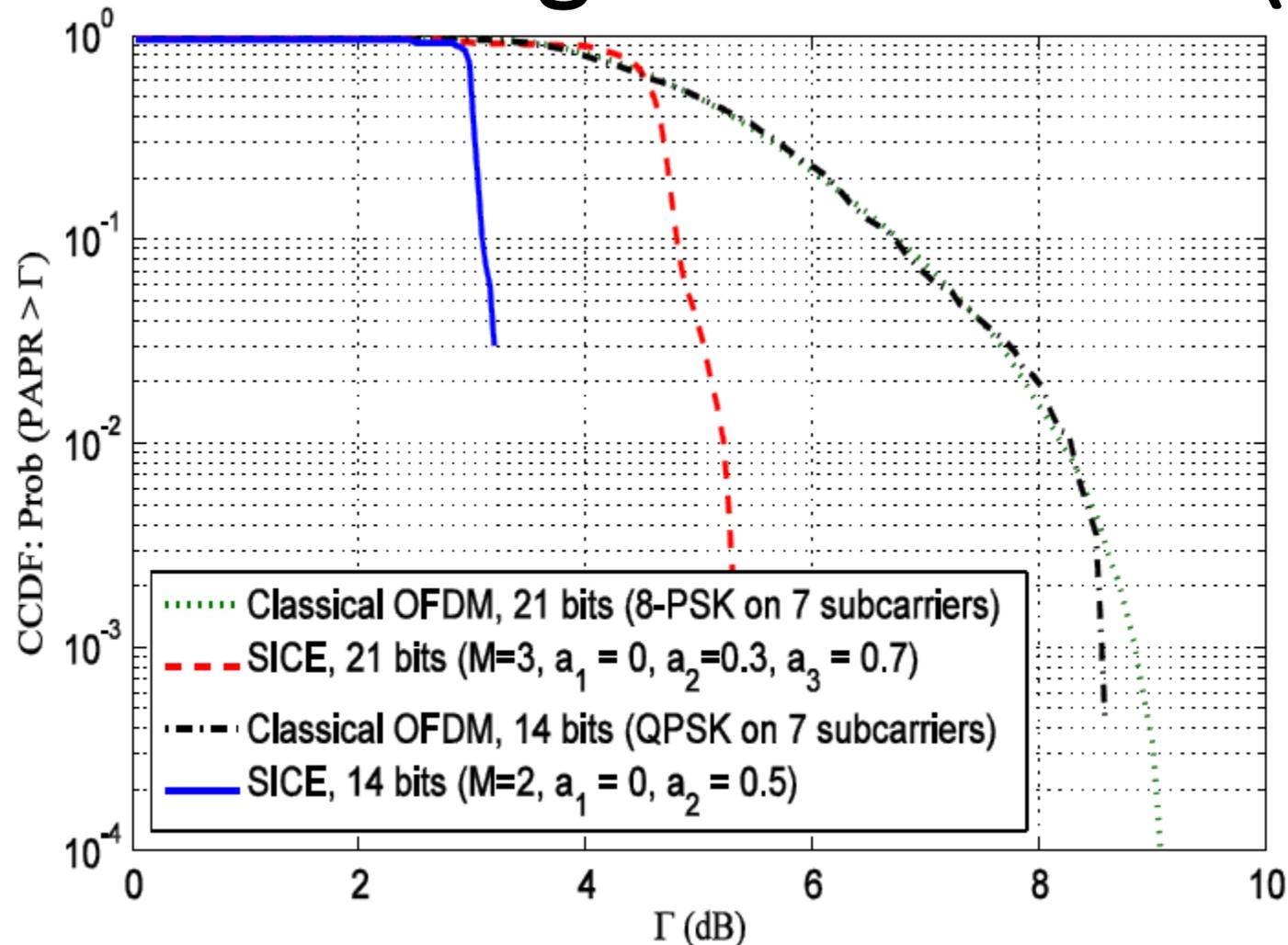
With SICE, the number of activated subcarriers is significantly reduced. As a result, SICE generally has a much smaller PAPR than conventional OFDM
