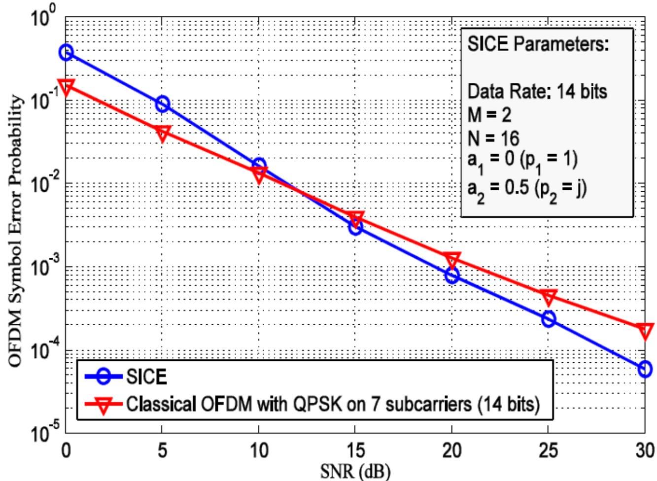
SICE outperforms conventional OFDM when the signal-to-noise ratio (SNR) is sufficiently high
