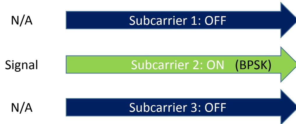
Information representation is also based on **WHICH** subcarrier(s) are used for signal transmission
