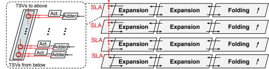
Fig. 6: Four physical slices, each implementing two expansion blocks and one folding block, are connected by TSVs which support SLA.
