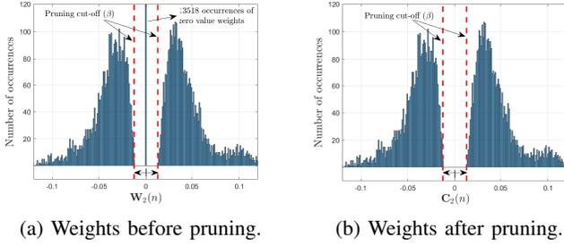
Fig. 8: Example of the weights compression by pruning applied to the second layer,  $\mathbf{W}_2(n)$ , of the baseline CNN detailed in Table III ( $\beta_k = 0.5 \times \sigma_k$ ).
