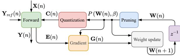
Fig. 9: Pruning followed by quantization iteration,  $P \rightarrow Q$  iteration, architecture.
