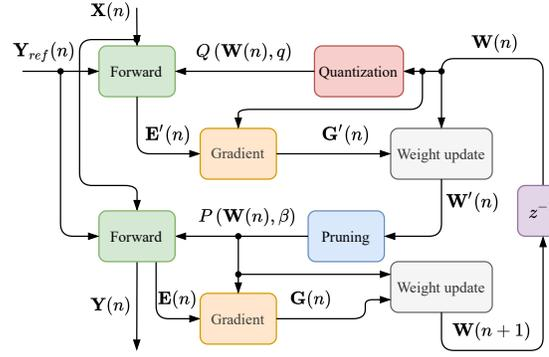
Fig. 11: Quantization followed by pruning iteration,  $Q \rightarrow P$  iteration, architecture.
