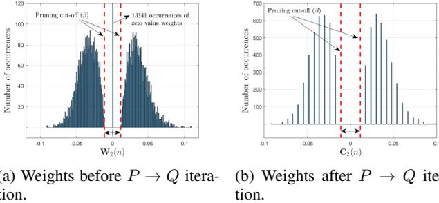
Fig. 10: Example of the weights compression by  $P \rightarrow Q$  iteration applied to the second layer,  $\mathbf{W}_2(n)$ , of the baseline CNN detailed in Table III. We assume,  $\beta_k = 0.5 \times \sigma_k$  and  $b = 5$  ( $M = 31$ ).
