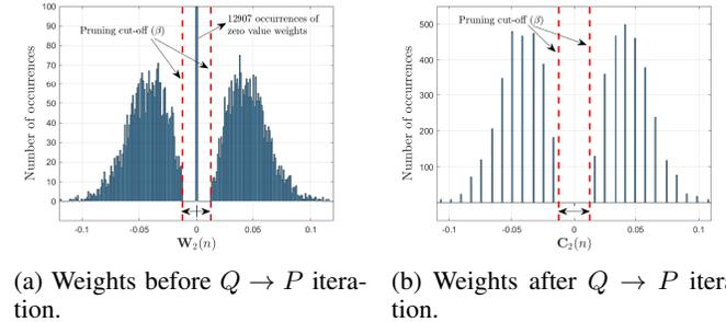
Fig. 12: Example of the weights compression by  $Q \rightarrow P$  iteration applied to the second layer,  $\mathbf{W}_2(n)$ , of the baseline CNN detailed in Table III. We assume,  $\beta_k = 0.5 \times \sigma_k$  and  $b = 5$  ( $M = 31$ ).
