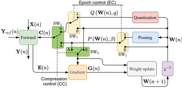
Fig. 21: Conventional scheme of pruning epochs followed by quantization epochs,  $P \rightarrow Q$  epochs, architecture.
