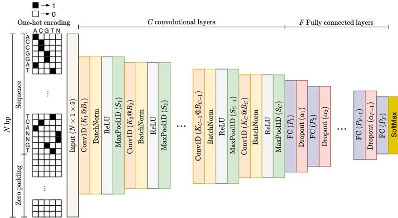
Fig. 3: One-hot encoding and CNN applied to a viral classification problem.
