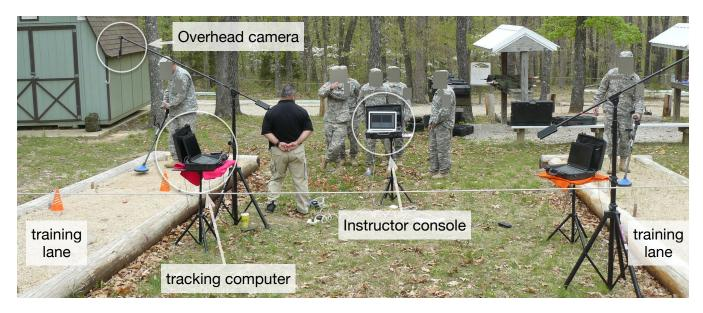
Figure 3: Deployment of Petals at HDTC. Segments of two neighboring lanes are monitored by overhead cameras. A tracking computer is dedicated to each lane. A centrally-located instructor console displays real-time visualizations of trainee performance from both lanes.
