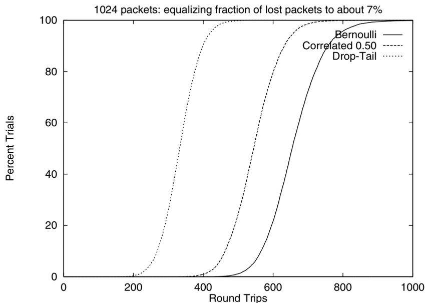
Figure 13. Cumulative distributions when overall packet loss percentages are equalized.
