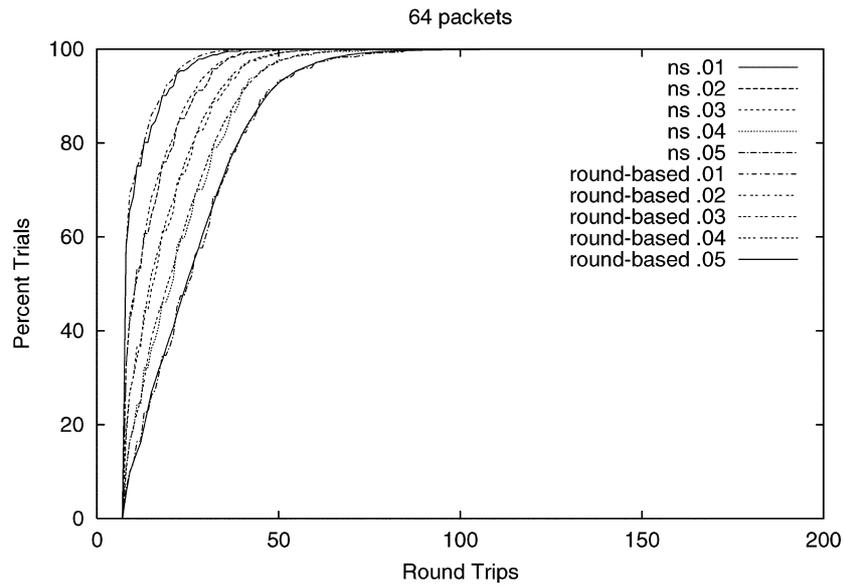
Figure 1. Comparison between ns and round-based simulations for the Bernoulli loss model with respect to rounds; 64 packets, packet loss 1–5%.
