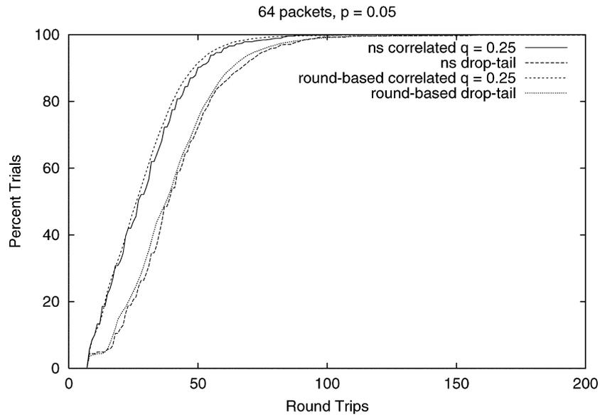
Figure 4. Comparison between ns and round-based simulations for the Correlated and Drop-Tail models with respect to rounds, 64 packets.
