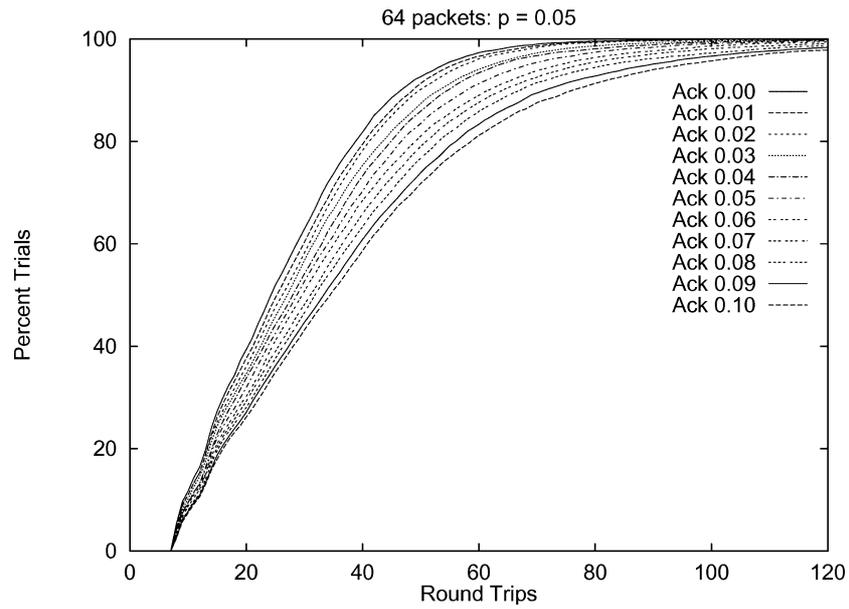
Figure 14. Cumulative distribution functions as lost acknowledgments increase: 64 packets.
