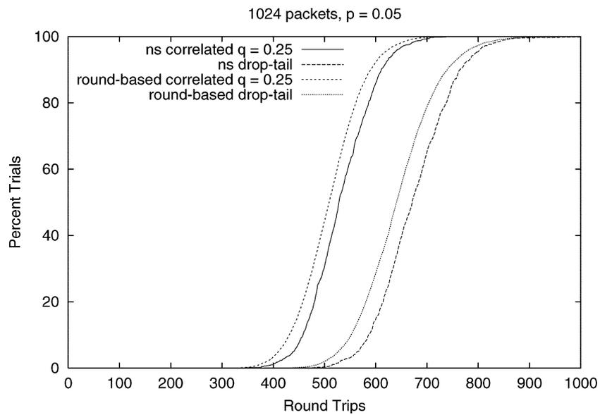
Figure 5. Comparison between ns and round-based simulations for the Correlated and Drop-Tail models with respect to rounds, 1024 packets.
