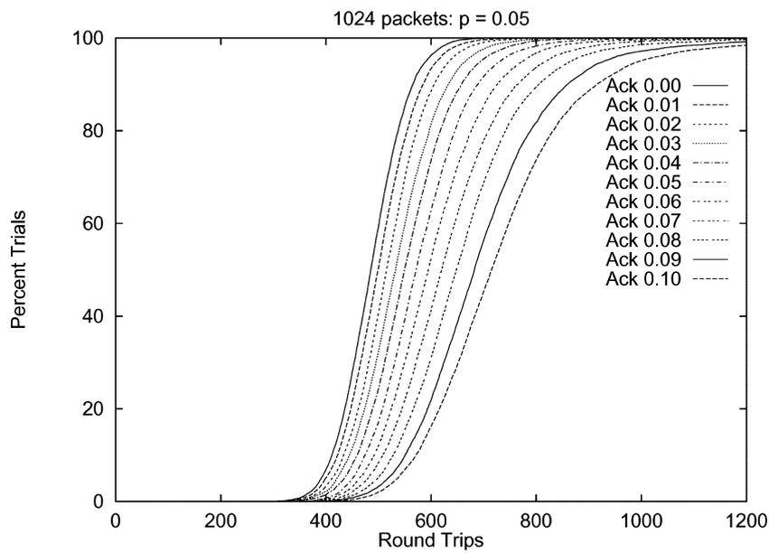
Figure 15. Cumulative distribution functions as lost acknowledgments increase: 1024 packets.
