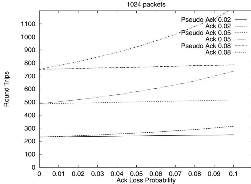
Figure 16. The effects of lost acknowledgments versus pseudo-ack loss.
