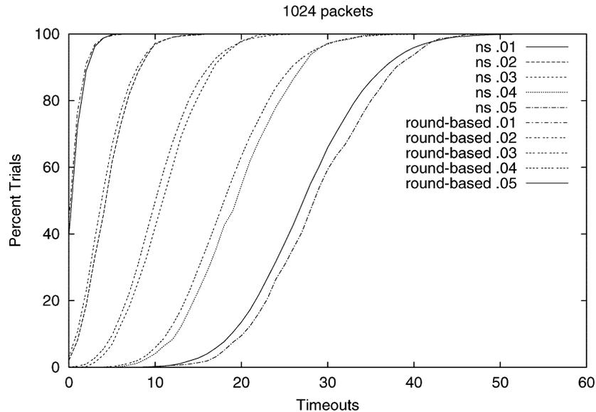
Figure 3. Comparison between ns and round-based simulations for the Bernoulli loss model with respect to timeouts; 1024 packets, packet loss 1–5%.
