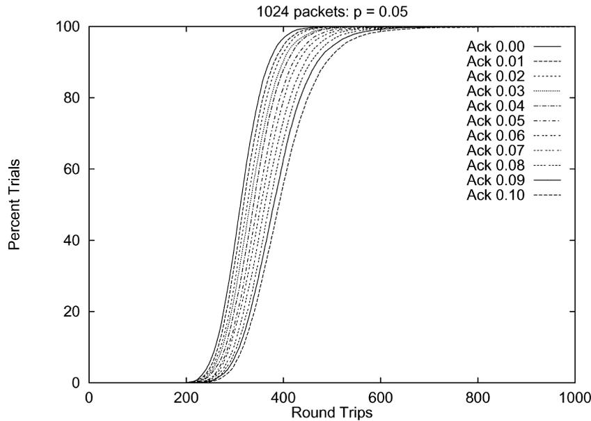
Figure 18. Cumulative distribution functions as lost acknowledgments increase without delayed acknowledgments.
