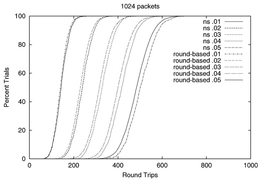
Figure 2. Comparison between ns and round-based simulations for the Bernoulli loss model with respect to rounds; 1024 packets, packet loss 1–5%.
